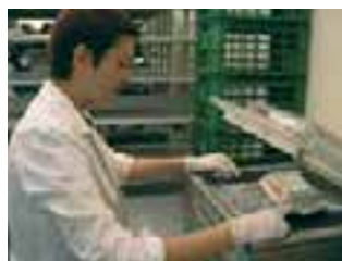
ArchiPress™ vacuum-packing machine in use for Squelch Drying flood-damaged materials
